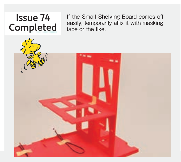
If the Small Shelving Board comes off easily, temporarily affix it with masking tape or the like.
